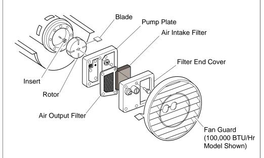
Figure 18 - Rotor Location
